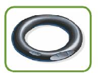
The seal or parts of the seal may exhibit small cuts, nicks or gashes. Sharp edges on the glands or components, improper sizing, or a low modulus/hardness elastomer may lead to installation damage.
