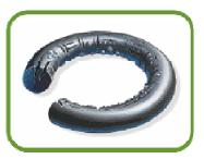
The seal exhibits blisters, pits, or pockets on its surface. Absorption of gas at high pressure and the subsequent rapid decrease in pressure results is gas that was once trapped inside the elastomer to explosively decompress and exit the seal. The absorbed gas blisters and ruptures the surface as the pressure is rapidly removed
