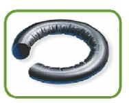
The seal may exhibit radial cracks located on the highest temperature surfaces. In addition, certain elastomers may exhibit softening, or a shiny surface as a result of excessive temperatures.
